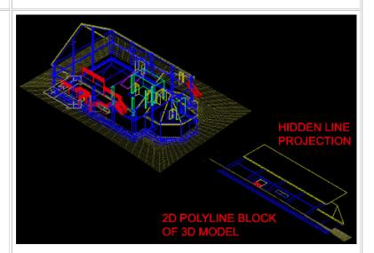
The resultant Projection is a regular **AutoCAD block** and can be exploded for editing. The block is made of polylines and usually the layers and colors come through okay. Once Exploded, you may find numerous redundant lines that require cleanup. Use the **Overkill** command from the Express Tools to remove extra lines. Notice, in the illustration above, that the 3D grade mesh was also transcribed by this routine; indicating its amazing ability to project
