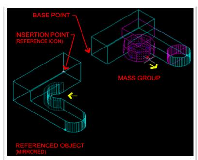
The Insertion point on the Referenced Object provides the only Grip editing point; thus behaving much like a common AutoCAD Block. Changes to the parent object reflect in the Reference once they have been completed.
