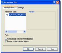
At times you may find that the default Design Content in ADT lacks a bit of design quality or is a bit off dimensionally. By using the **RefEdit** tool, you can make fairly short work of modifying Multi-View Blocks. You can employ this technique to any MvBlock in your current drawing or Open the original source file, RefEdit it and then save it for a permanent change to your library.
