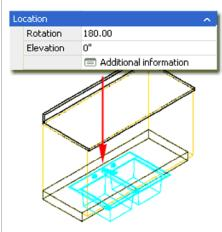
On the **Location** tab of the **Multi-View Block Reference Properties** dialogue box, you will find Insertion Point value fields that you can use to adjust the position of a Multi-View block should its default Insertion Point prove to be
