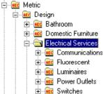
Note: When Electric Fixtures, like the Fluorescent Lights, are dragged in from the DesignCenter, make sure to use the "Select Lavout Node" option to Anchor the fixture to the Ceiling Grid object. You should find this comment stated on the command line once the fixture has been dragged in. If you ignore this option, you will not be able to Mask with the fixture nor take advantage of the Anchoring features that save a lot of time in labor. To repair a lost Anchor use the Node Anchor tool
