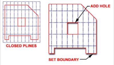
**Set boundary** - use to define a new perimeter shape for your column grid. To remove, delete the boundary polyline. Keep the boundary polyline on a separate layer if you want the option to turn it off separately from the grid.
