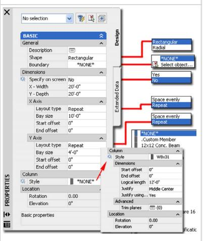
**End offset** - an amount of distance from the grid object's end that you want the actual grid to end at. This does not affect Spacing but it does affect overall X-Width.
