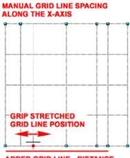
Once a Grid Object has been set to "Manual", you can use the Bays dialog box to Modify Spacing and Add/Remove Grid Lines. You can also use the Context Menu, illustrated above left to Add or Remove Grid Lines. In addition to using the Bays along X Axis or Bays along Y Axis dialog boxes for exact numeric distances for Grid Lines, you can use Grips to Stretch and position Grid Lines as you need.
