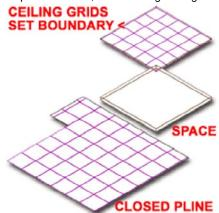
origin and then a second corner for the overall rectangular grid space; i.e, you can add a ceiling grid one grid at a time. The grid will be limited by the proportions specified by the X-Baysize and Y-Baysize. Or, if you use the Divide By method, the grid will constantly be divided up to match the Divide By number.
