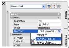
The **Clip Column Grid** tool may not prove to be as useful as the Clip Ceiling Grid tool but they work the same way. Since a Column Grid begins as a rectangular or circular shape this is the only way to modify it to match an irregular plan design.
