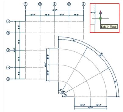
If you use the "**ColumnGridDim**" command, however, you will be able to produce automatic dimensions in all four directions simultaneously - even on radial grids. Once you select this command, you will be prompted for the distance you want your dimensions away from the closest grid line. The Style is based on the current Dimension Style - DDIM. The disadvantage of using this option is that you don't get Aec Dimensions but simply regular AutoCADlike Dimensions.
